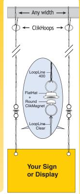
Keeping the Pole vertical, extend it to the FlatHat height. Attach one ClikMagnet to the metal in a FlatHat, then walk to the next FlatHat location and repeat. Clik-Clik—Your Sign is Hung!
